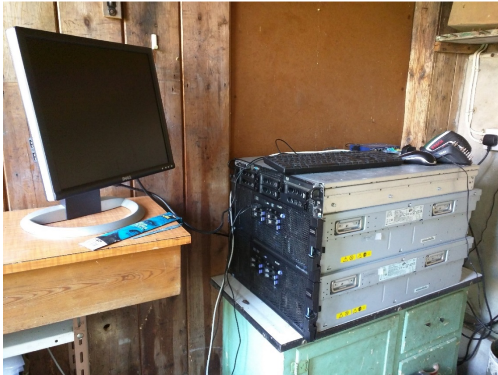
Figure A8-1 – ‘Shed-hosted’ personal Private Cloud (1*2U Dell PowerEdge 2950, 2*4U IBM System x3850 M2)
